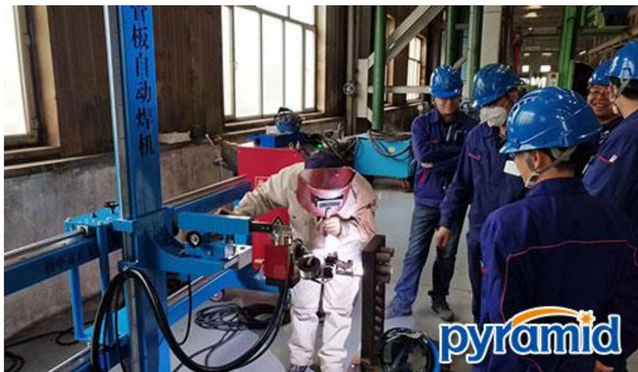
The deep hole welding machine can be used for the inner hole wire flat welding and wire fillet welding of air cooler, and can also be used for the inner hole lap welding, inner hole butt welding and back butt welding of pipe tube plate.
