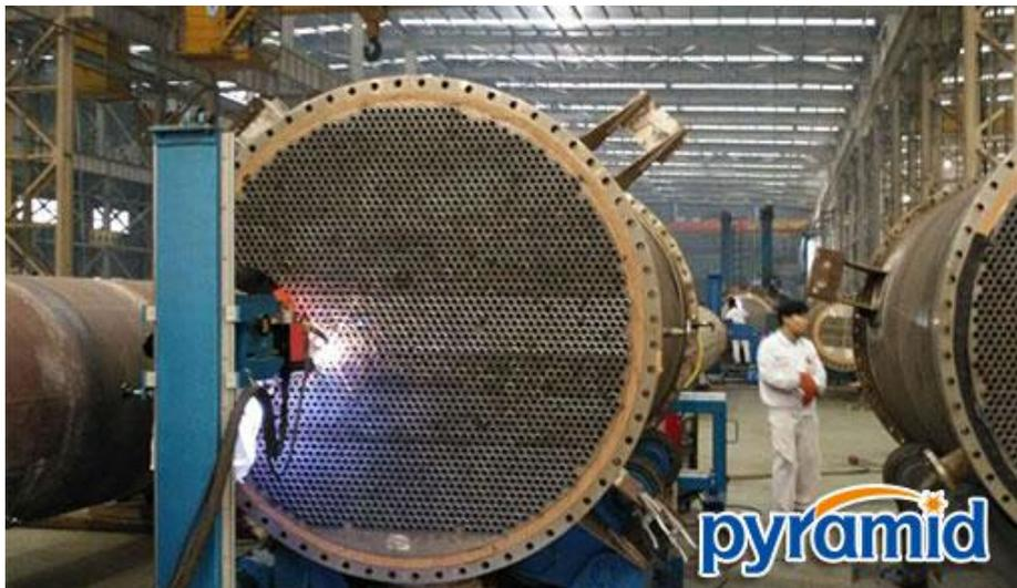
This machine adopts the PLC produced by Siemens to control and installs the software developed by our factory. The whole welding process is automatically completed according to the preset procedures and processes.
